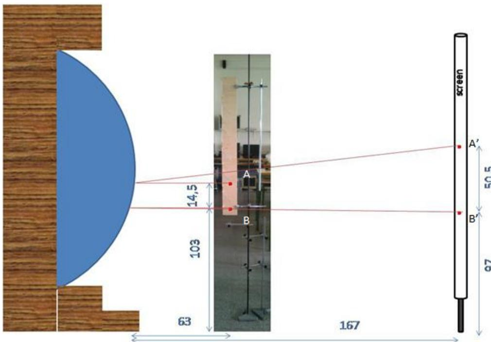
Image 3 Representation of the “Reflexeitor”, the convex mirror and the screen with their measures.
