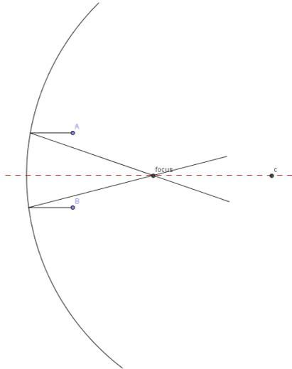
**Image 6** Representation of the beam's direction.
