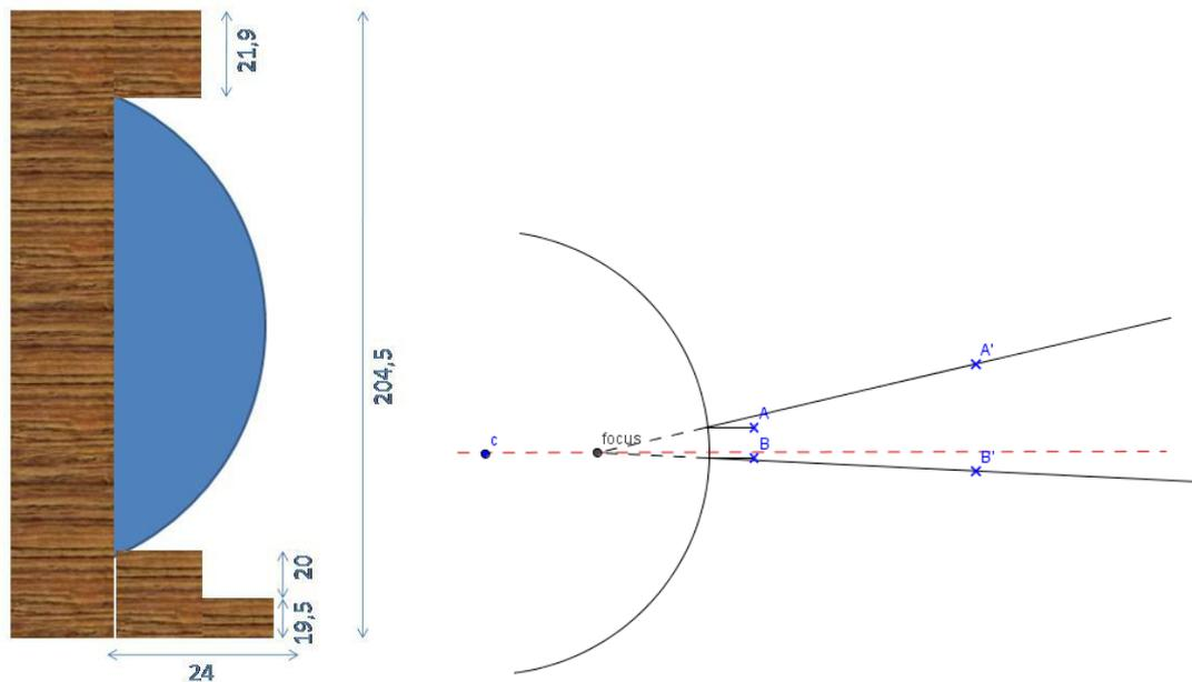
Image 4 Measures and beam's direction.
