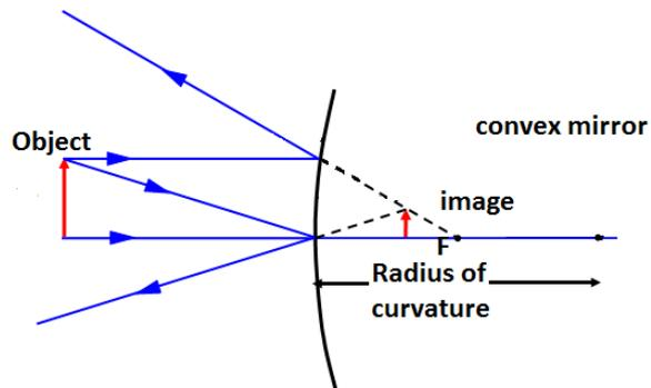
Image 2 Graphical representation of a convex mirror.
